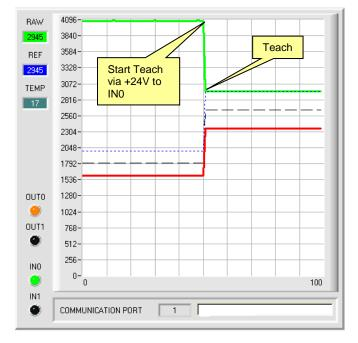
RAW 4096 3840-2527 IN0 turns to LO 3584 -REF MAX 3328-3212 3072-TEMP 2816-17 2560 MAX 2304-3212 IN0=HI 2048 MIN 1792-2020 1536 OUTO 1280 0 1024 OUT1 768 9 512 256 INO 0-0 9 100 IN1 COMMUNICATION PORT ø
