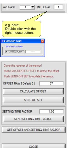
Offset calibration can be accessed by double-clicking with the right mouse button exactly at the frame below **INTEGRAL** in the **PARA** tab.
