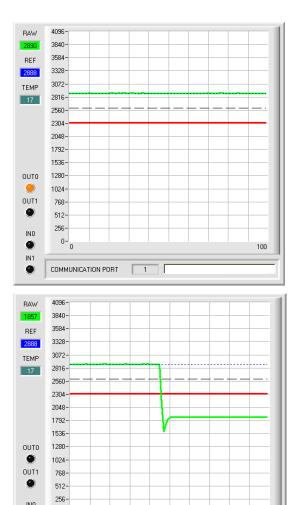
As long as the current measurement value RAW (green line) lies above the switching threshold (red line), the output OUT0 has +24V (signal is OK). This is visualised by the **OUT0** LED.
