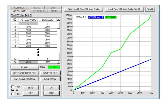
When the GO button is pressed the current RAW value is shown in the RAW display.
